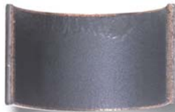
Incipient delamination (Standard material)
